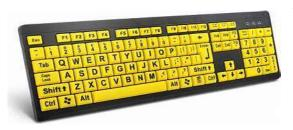
A keyboard has many buttons which are called keys. Each key has a letter, a number or a symbol written on it. It is used for typing letters, words, numbers and special symbols. There are 104 keys present on a standard keyboard.
